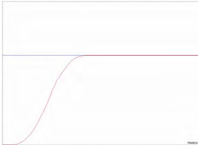
Figure 26: Response to a system tuned with the method of Ziegler and Nichols
